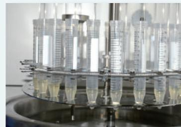
3. Concentrate by 24-Well Plate Intelligent Nitrogen Evaporator
