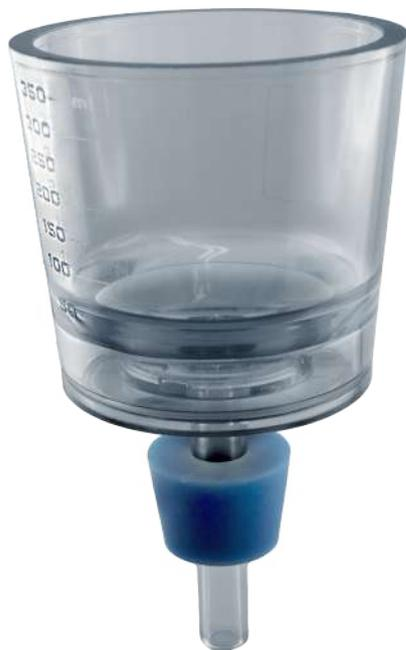
The GVS polysulfone 47 mm autoclavable filter holder combines the Gravi-Seal filter holder uses a unique gravity held design that allows for one-handed operation with no danger of filter by-pass or sample leakage even when using depth filters.
