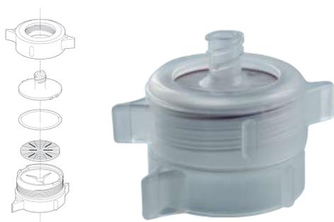
The GVS polypropylene 25 mm filter holders are very useful for ultra cleaning and sterilizing small volumes of liquids from a syringe. Due to the polypropylene construction, they can be used over a wide temperature range with excellent chemical compatibility. In the case of the syringe, the inlet cap locks into the base to prevent twisting damage to the membrane as the cap is tightened. Projection lugs on the base and the cap allow these units to be assembled and sealed quickly and efficiently.
