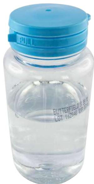
Prefilled sterile dilution bottles are designed for sample dilution of water, dairy products, foods, and pharmaceuticals prior to microbiological testing. Final pH for all solutions is 7.2 pH  $\pm$ 0.2 pH at 25°C. They come in an easy open, flip-top, plastic container with a tamper-evident seal.
