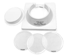
GVS Life Sciences PM 2.5 PTFE Membrane is a high-purity, thin membrane for PM 2.5 ambient air monitoring. Each membrane is sequentially numbered with a chemically resistant polypropylene support ring. The low tare mass allows for accurate gravimetric determinations. No glues or adhesives are used in making the membranes and its stable design eliminates curling, keeping the membrane flat allowing for robot use.
