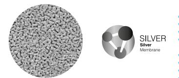
Silver membranes are composed entirely of 99.97% pure metallic silver. They provide excellent chemical resistance and high temperature characteristics. Orientation of the membrane can be important. There is a distinct difference in surface characteristics with one side appearing shinier than the other. Use the Shinier side upstream for scanning electron microscopy. For all other applications and analytical work use the duller side upstream.
